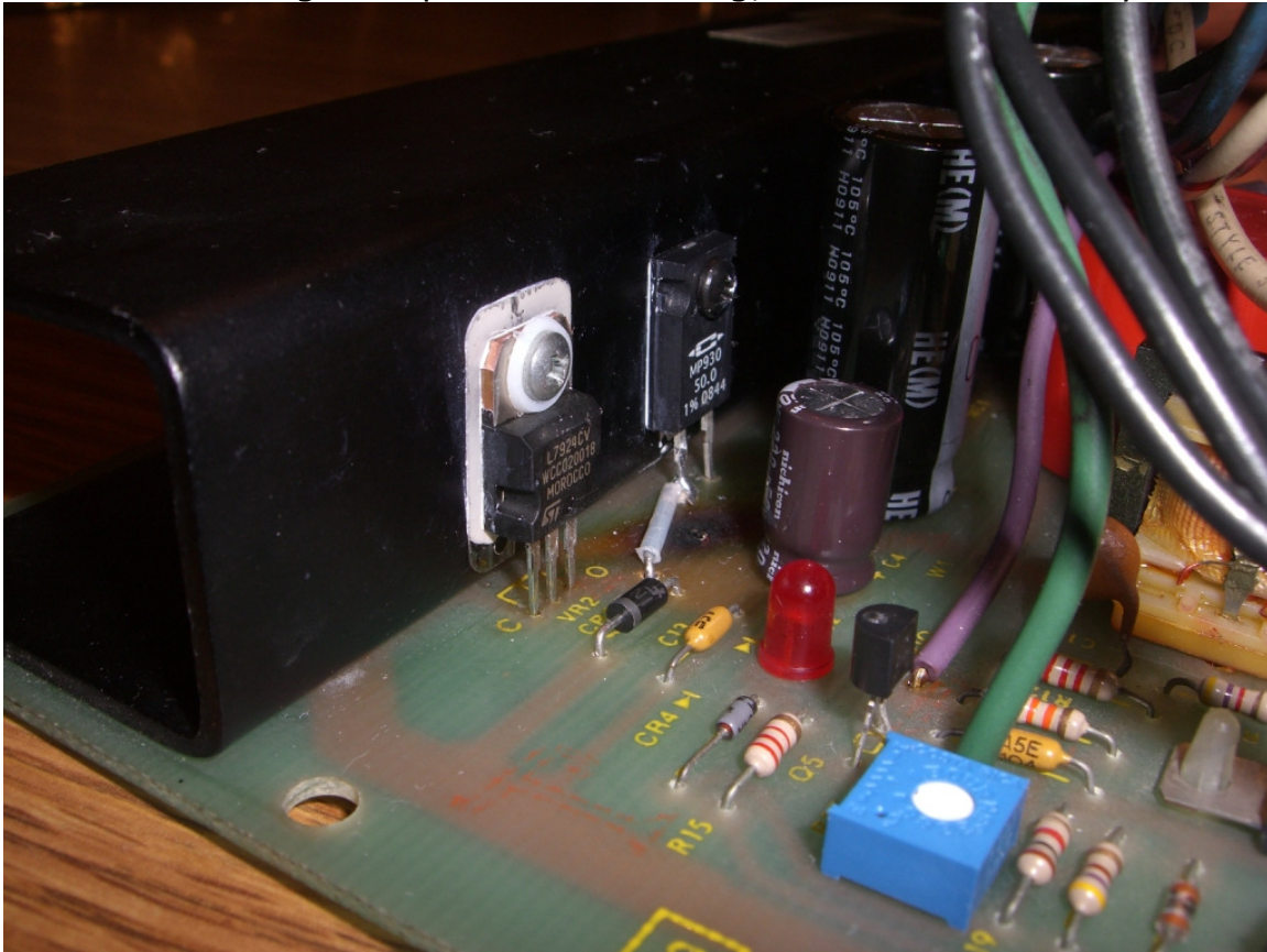
Figure 2 Power Resistor (Right of VR2)
